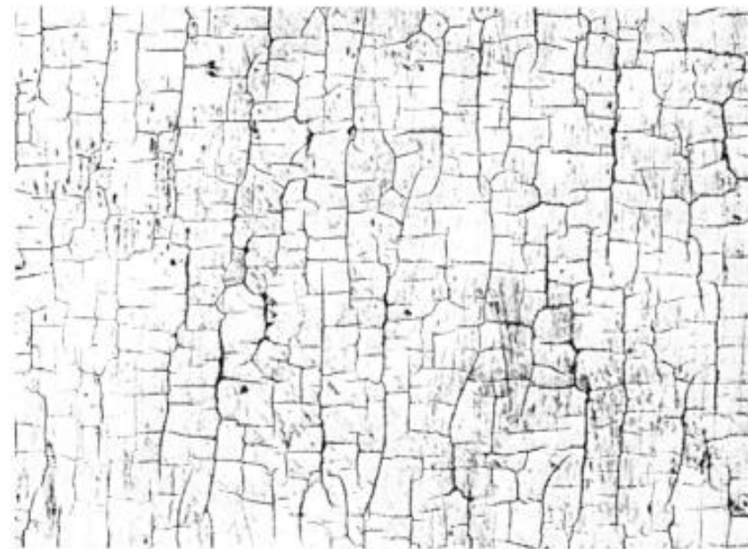
Figure 2 Example of a craquelure pattern showing cracks PARALLEL to the wood grain; Flemish; Hieronymus Bosch, 'Christ Mocked'. Horizontal dimension 4.5cm.
